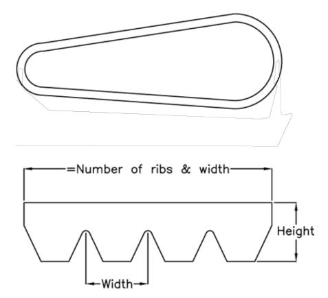
$\begin{array}{ll} \text{Datum Llength} = 1651 \\ \text{Height} &= 3.5 \\ \text{Number of ribs} = 7 \\ \text{Pitch} &= 2.34 \end{array}$
